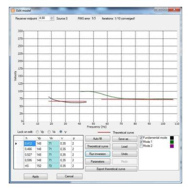
As you can see, no curve fitting was performed (the curves remain unchanged). This is due to an ineffective initial model that caused the inversion to "drop" into the local minimum. To solve the problem, we need to select another (more appropriate) initial model for the inversion procedure.
