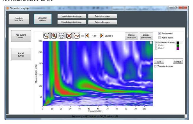
The next step is to "extract" the dispersion curve by means of picking the image by amplitude maximums. In this example we will describe the process of generating the transverse velocity section using not only the principal mode, but also the first higher mode which is clearly visible in our case.
