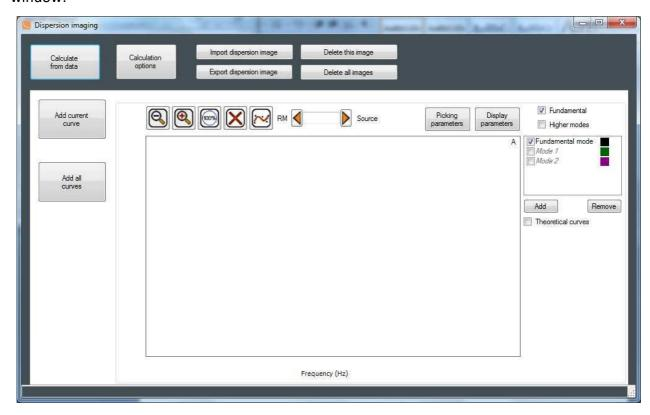
To calculate the dispersion images, press the **Calculate from data** button, select the path to the previously saved **geom\_data** dataset in the database, and press **OK**.
