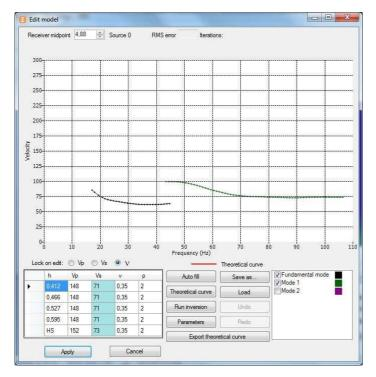
The initial medium model based on the previously specified parameters is shown in the lower part of the window. To display the theoretical curves for this model, press **Theoretical Curve** – they will be shown in red:
