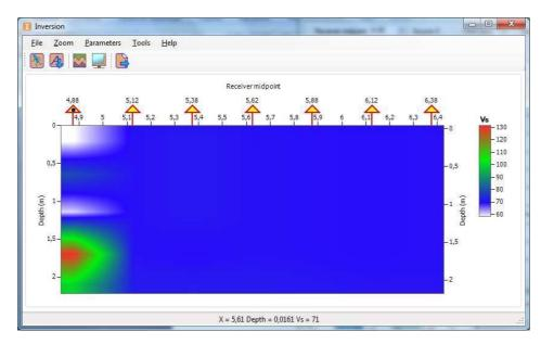
As was mentioned earlier, the curve fitting process depends heavily on the initial model selection. Therefore, let us proceed as follows: distribute the model generated at the first SP to all other SP to use it as the initial model.
