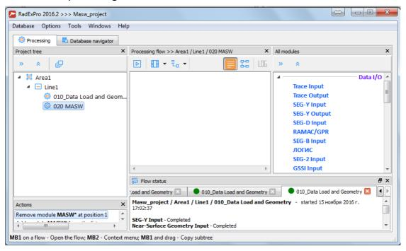
Open the flow and add the **MASW** module from the **Surface Wave Analysis** group. Data are processed within a processing scheme. A scheme is a combination of dispersion images, corresponding curves, the resulting model, and image and model calculation and visualization parameters. Each scheme is stored in a separate **MASW** directory within the project.
