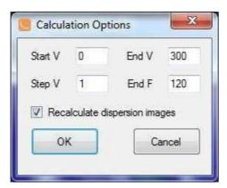
The **Recalculate dispersion images** option allows calculating the dispersion images immediately after pressing the **OK** button. When the new images are calculated, a message prompting to replace the old dispersion image for each SP will appear on the screen. Replace all images in the dataset by pressing **Yes to all**.
