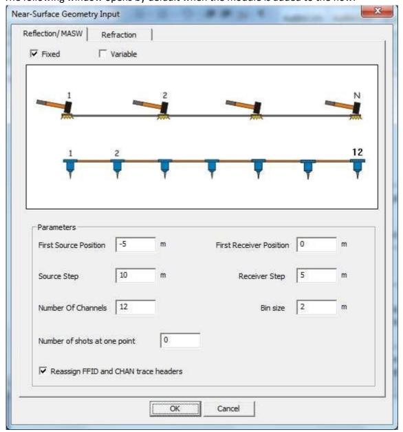
To assign geometry to the source files, you need to complete the following module fields according to the *survey parameters*: receiver line -24 channels, distance between the channels -0.25 m (vertical geophones). Distance between the source and the first receiver -2 m. The entire array was moved with 0.25 m increments (end-on shooting).
