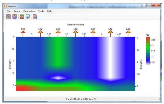
The triangles reprsent array midpoints associated with curves and, therefore, transverse velocity profiles. Enter the curve fitting mode by double-clicking the first SP triangle with the left mouse button.
