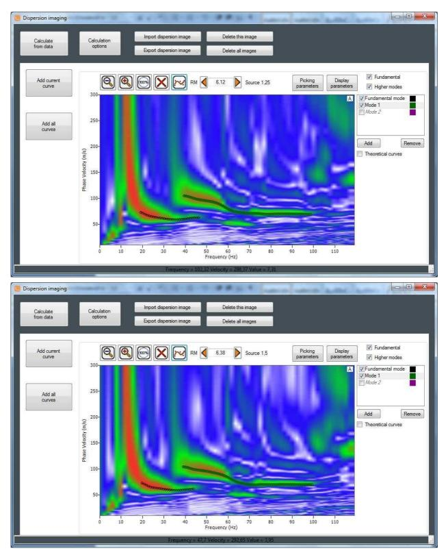
After all curves are picked, they need to be added to the list of curves to be processed (input into the inversion procedure). To do this, press **Add all curves** in the left part of the dispersion imaging window. The curves will appear in the list in the main project window:
