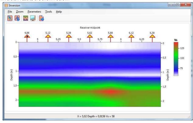
To verify the curve fitting quality for any SP, double-click the triangle corresponding to that SP. This will open the fitting window for that curve.
