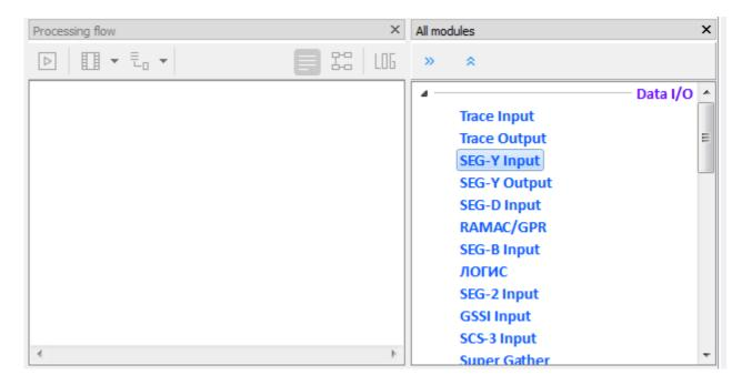
Let us create a flow consisting of the **Seg-y Input**, **Near-Surface Geometry Input** and **Trace Output** modules. The following procedures will be performed as a result (in the order they appear in the flow):
