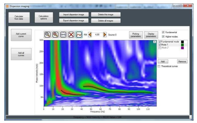
! Identification of both the principal mode and the higher modes on a dispersion image is not always a simple and clear procedure. In case of the principal mode it may be complicated by prevalence of higher modes as well as a fairly wide maximum in the lower frequencies. It should be kept in mind that changing the picking within relatively small limits may cause a substantial deviation of velocities in the resulting model.
