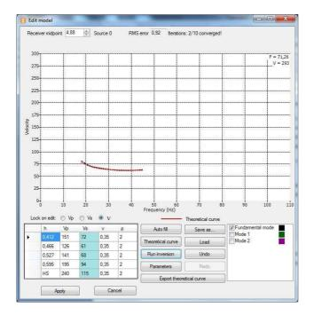
Now let us enable the higher mode and run the process once more. It means that this time we will be using the initial mode obtained by applying inversion to the principal mode to invert both modes. As you can see, with this approach the inversion was completed successfully, the curves were fitted, and the transverse velocity model was updated bases on the results of combined fitting of both modes.
