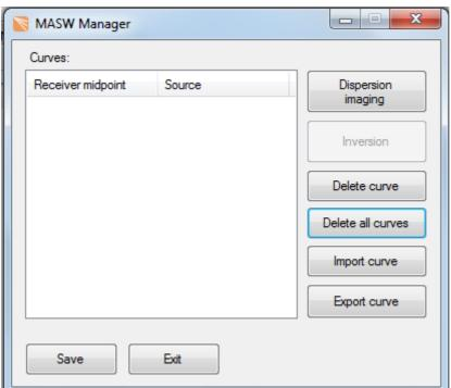
Launch the module by pressing the **Run** button. The main project management window – **MASW Manager** – will appear. The left part of this window shows a list of all dispersion curves that have been added to the scheme. The curves are sorted by the receiver array midpoint. The source coordinate (header SOU\_X) corresponding to the array midpoint coordinate is also
