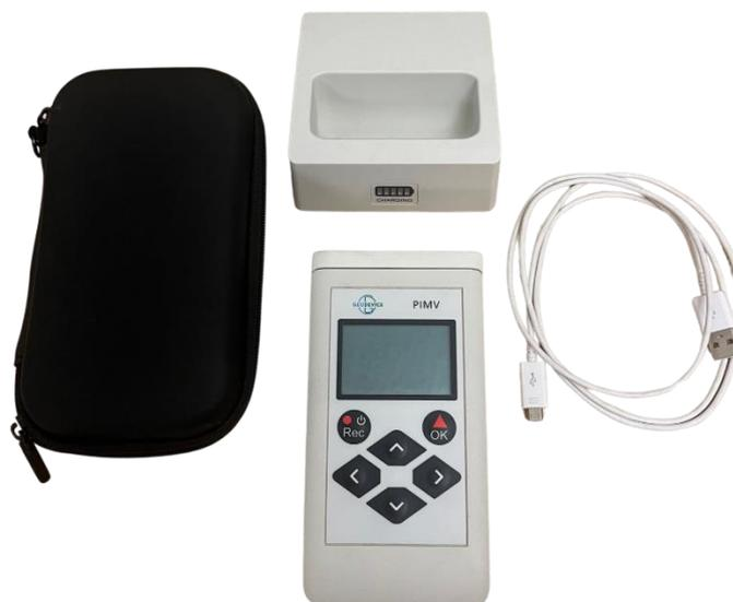
Figure 1 PIMV — portable magnetic susceptibility meter
