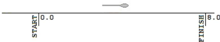
5. Press ACTION button at track ending (8.0 m position) to finish continuous measurement.
