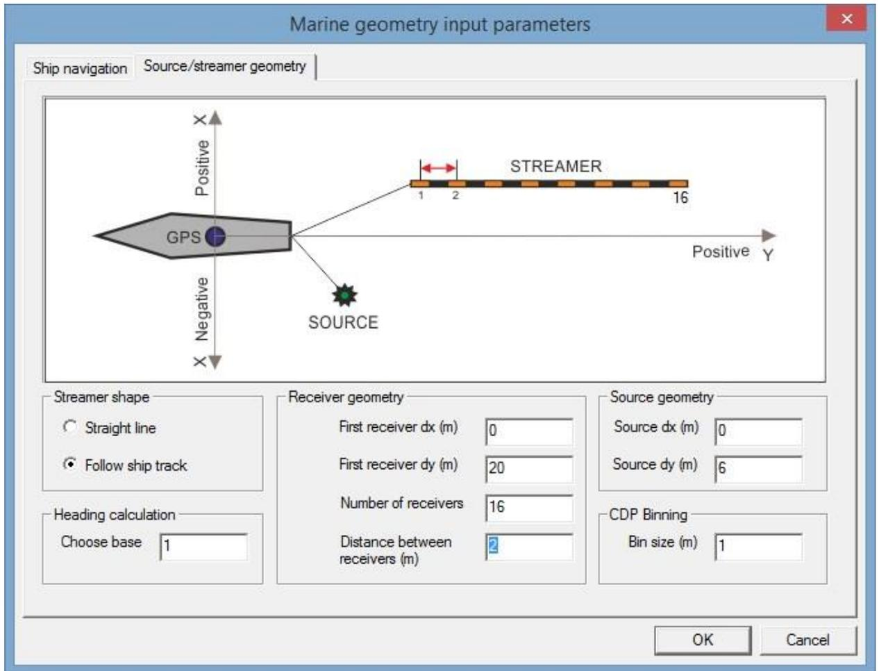
When you click on a geometry parameter here, it will be high-lighted on the scheme. We specify that our 16-channel streamer with 2 m channel spacing was towed 20 m behind the ship GPS antenna. The source was towed 6 m behind the antenna (which gives us 14 m offset of the nearest channel). Both the source and the streamer were towed on the same line with the GPS antenna (otherwise, we would like to define their side offsets, indicated as dx, as well).
