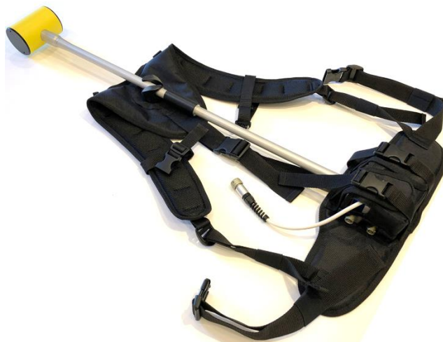
Figure 6 – Magnetometer and battery in the backpack harness
