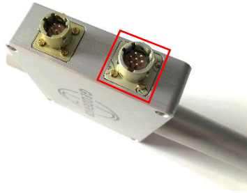
Figure 7 – Connector for a communication cable on the magnetometer case
