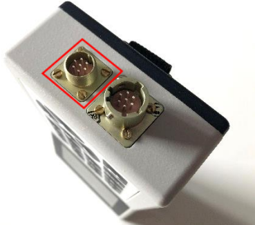
Figure 42 – Connector for USB cable on CU case
