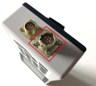
Figure 11 – Connector for connecting cable on the CU case
