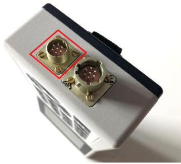
Figure 13 – Connector for connecting a cable with a remote start button on the CU housing
