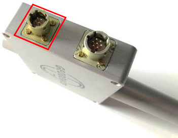
Figure 9 – Battery connector on the magnetometer case
