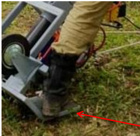
Figure 15 Location of the operator's foot on the base of the Accelerated weight drop
