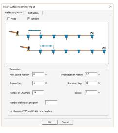
For more complicated survey designes you can load true positioning from SPS-files or ASCII tables.
