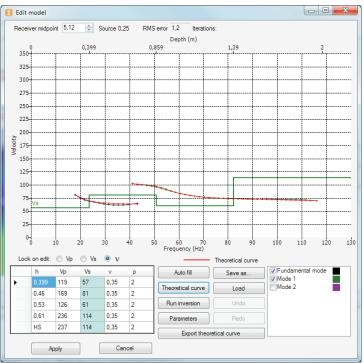
You can invert all dispersion curves automatically with a single mouse click, or work thoroughly with each curve one by one with your complete control of everything. You can also use the inversion result of one midpoint as the initial model for automatic inversion of the others.
