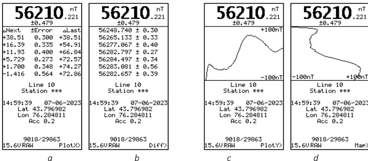
Figure 69 Found data window with different modes of displaying
