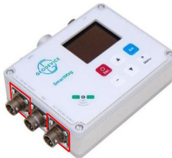
Figure 115 Battery connector on SmartMag electronics unit
