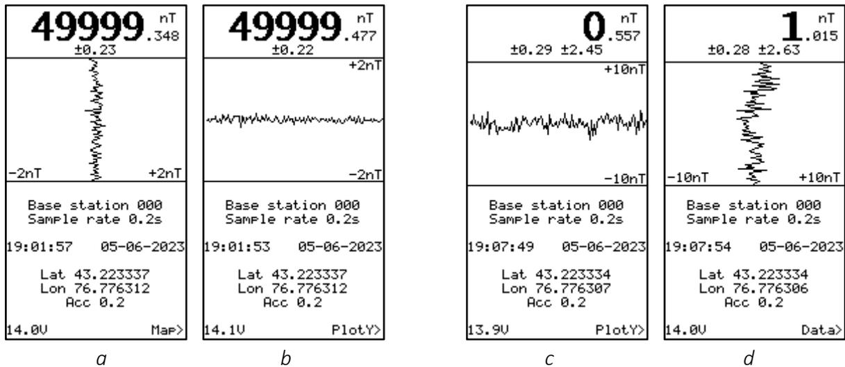
Figure 63 Window with a graph of measurements in the Base station mode
