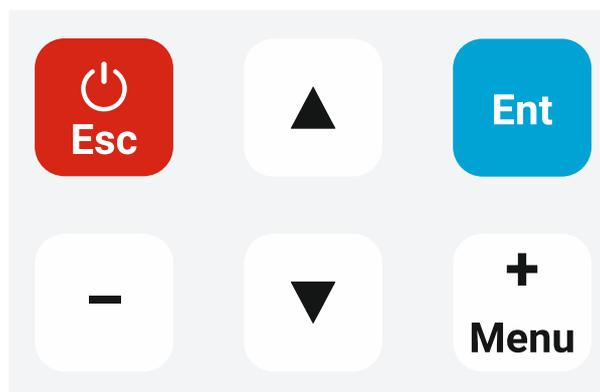
Figure 82 Main keypad of the console of SmartMag Overhauser magnetometer
