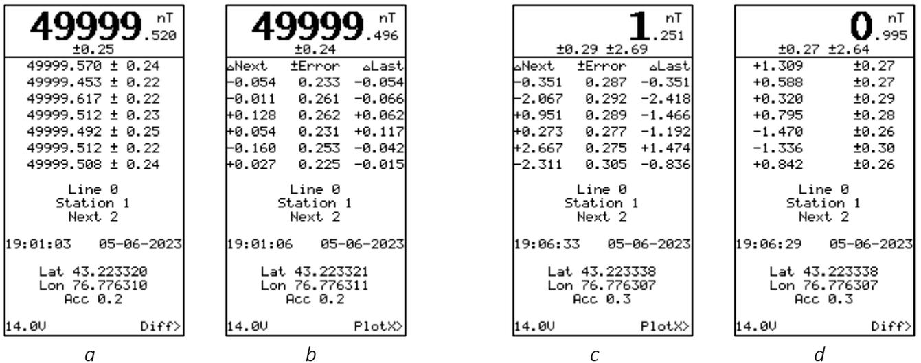
Figure 56 Measurement window in the Mobile survey mode
