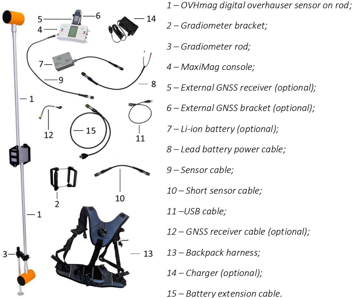
Figure 3. OVHMag set on rod in gradiometer configuration
