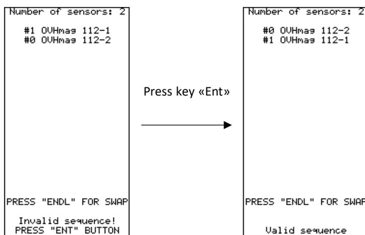
Figure 71 Gradiometer Sensor list window
