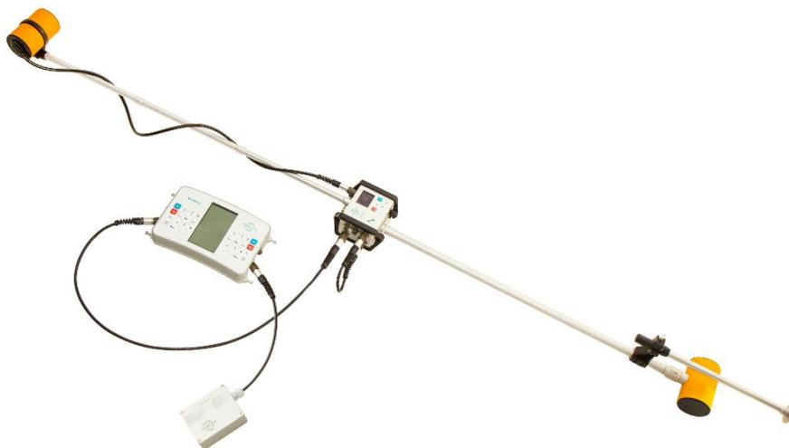
Figure 36 OVHmag-SmartMag magnetometer-gradiometer assembled
