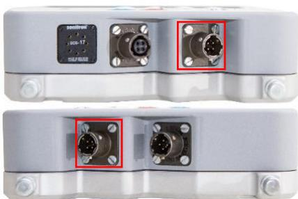
Figure 114 Battery connector on MaxiMag console
