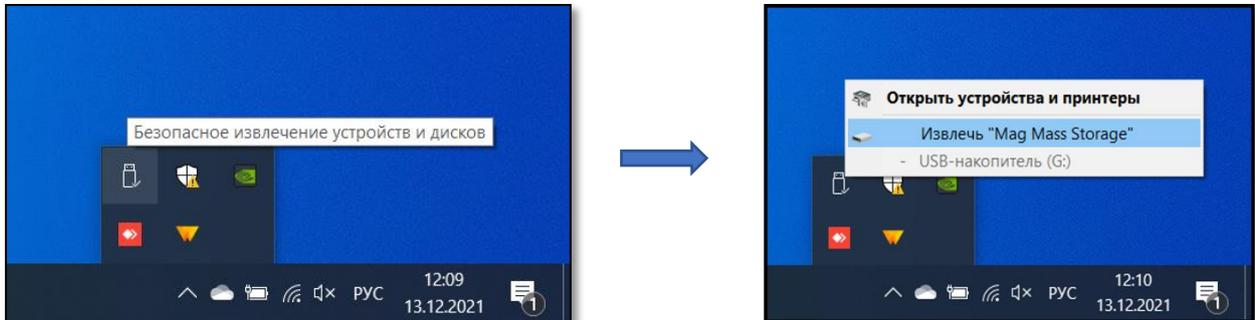
*Figure 134 Safely Remove SmartMag Hardware*
