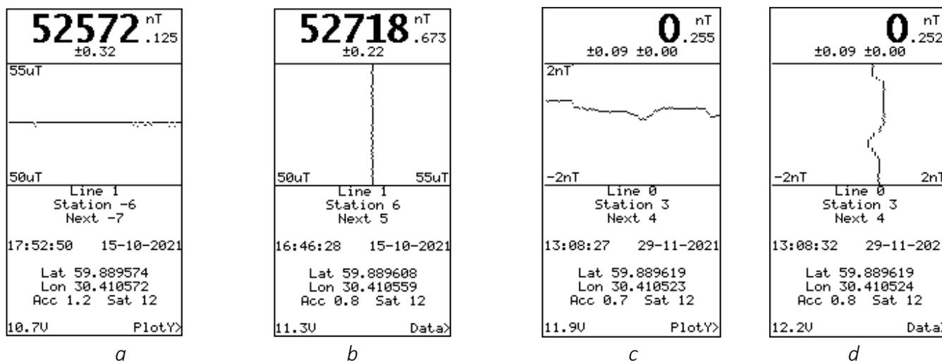
Figure 59 Window with a graph of measurements in the Mobile survey mode
