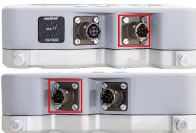
Figure 120 CAN FD or RS-232 cable connector on MaxiMag console
