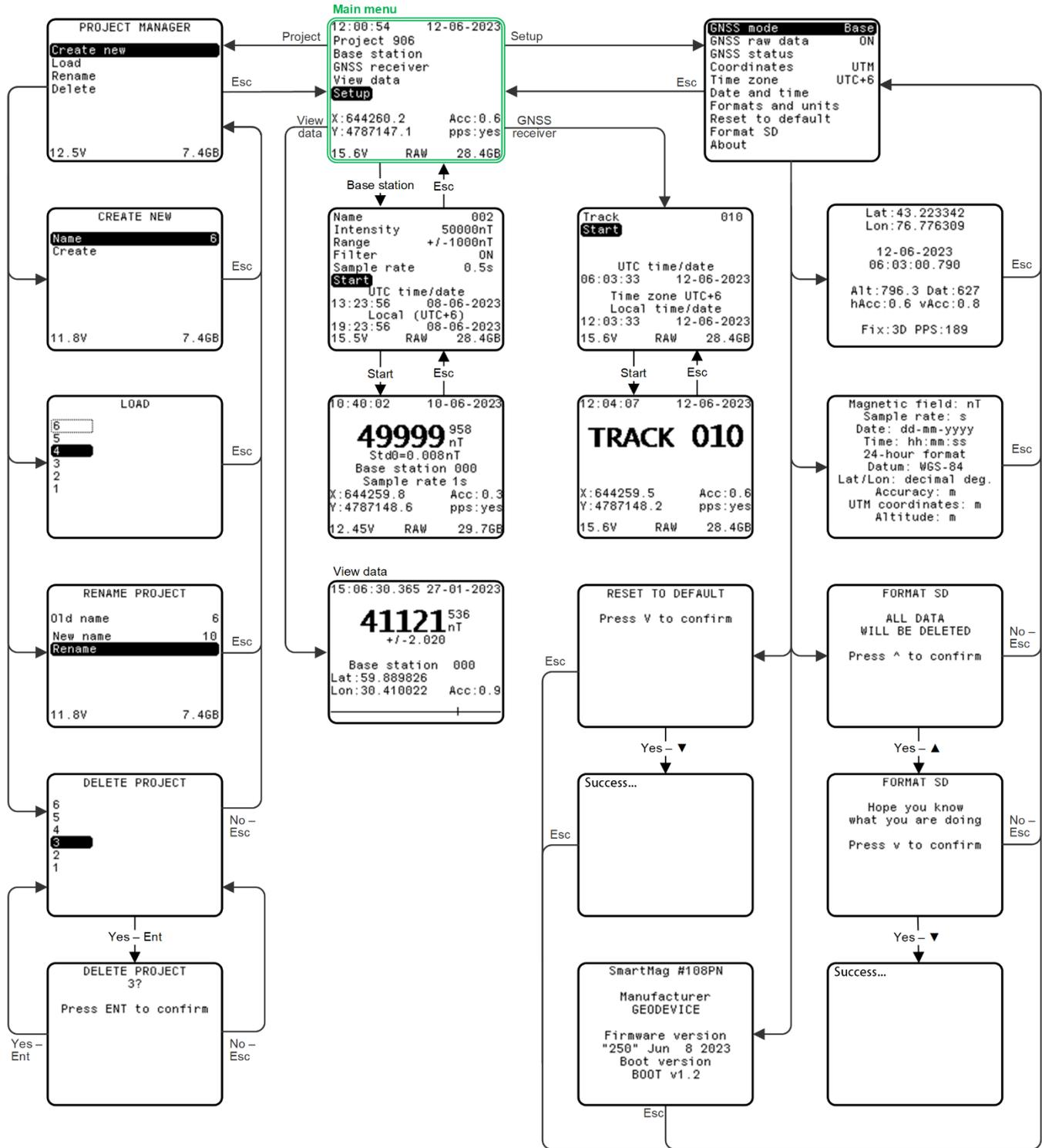
Figure 93 Commands control of the SmartMag Overhauser magnetometer
