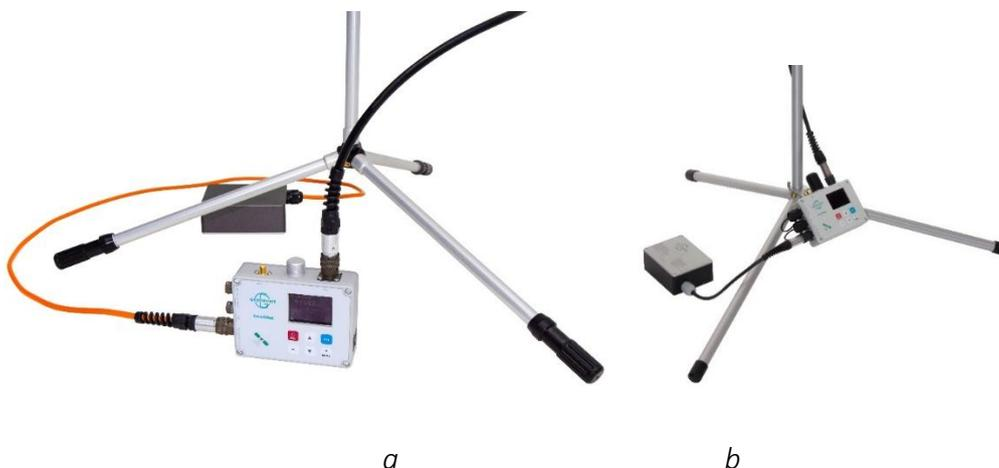
Figure 90 Console with the Overhauser sensor and battery
