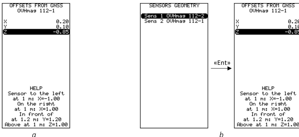
Figure 72 Offset from GNSS receiver geometry setting
