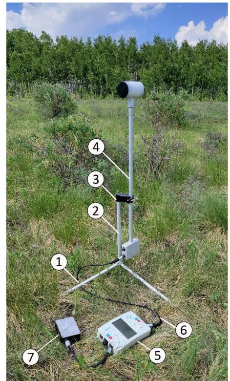
Figure 40 MaxiMag as a base station
