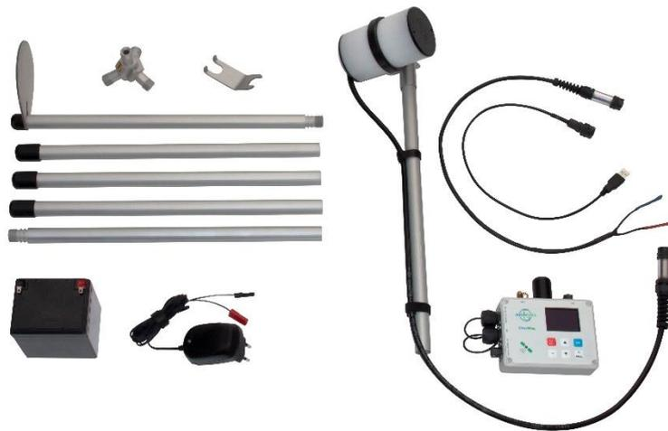
Figure 4 SmartMag Overhauser magnetometer
