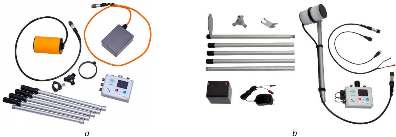
Figure 81 Components of SmartMag Overhauser magnetometer
