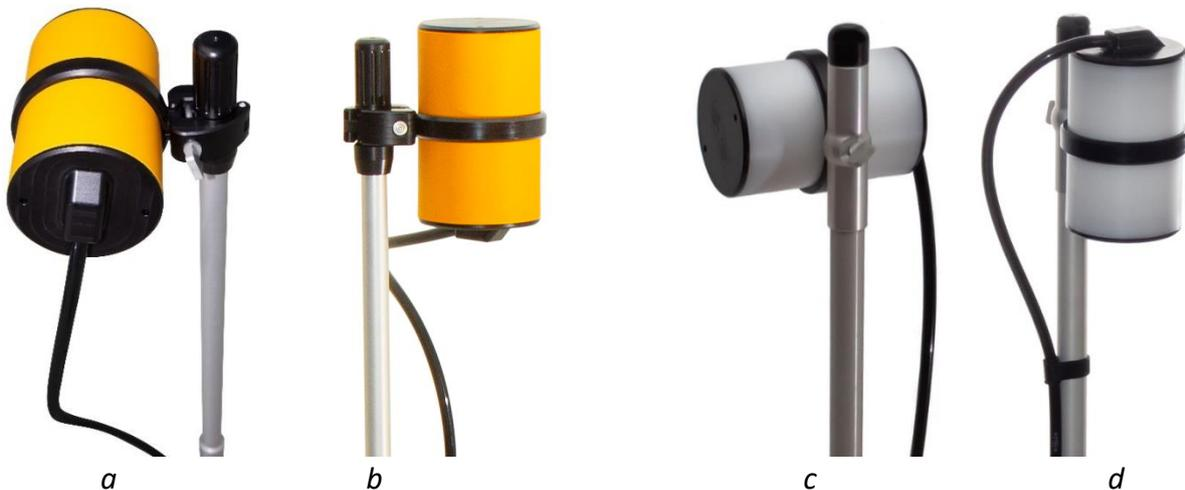
*Figure 85 Overhauser sensor fixed on the non-magnetic tripod*
