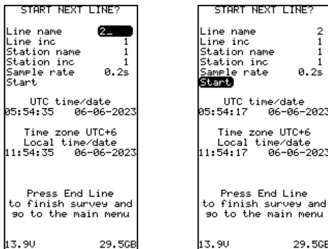
Figure 58 Start menu window for measurements on the next profile
