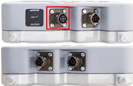
Figure 25 GNSS connector for GPS cable connection to console
