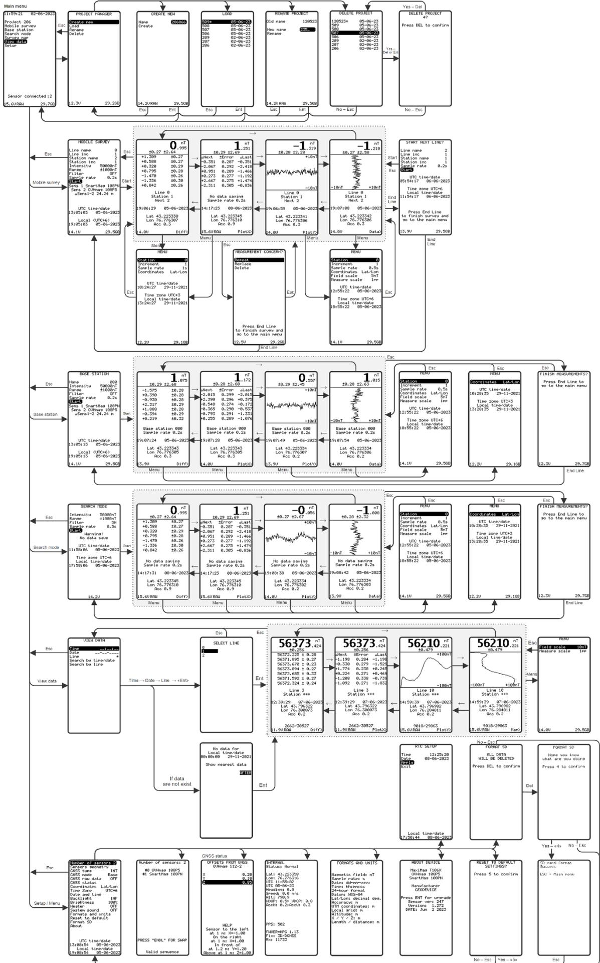
Figure 12 Commands control of the MaxiMag Overhauser gradiometer (2 or more sensors connected)
