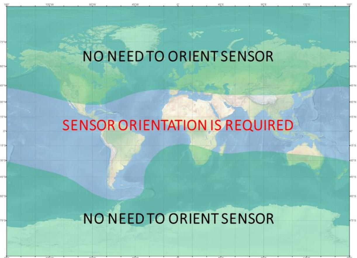
Figure 44 Map where the Overhauser sensor has to be oriented
