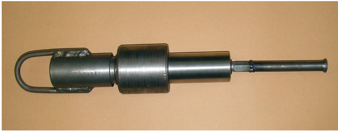
Figure 10 Source head with the cartridge chamber
