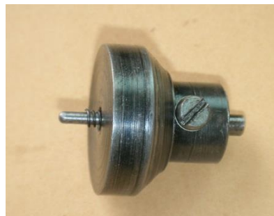
Figure 7 Striking pin assembly
