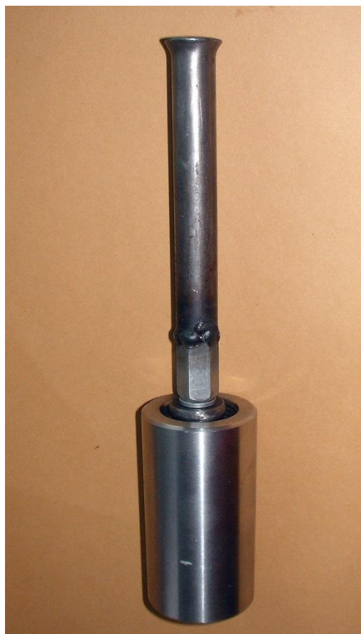
Figure 9 Striker's tube and striker with guide tube
