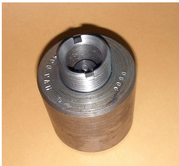
Figure 8 Receiver with striking pin and clutch
